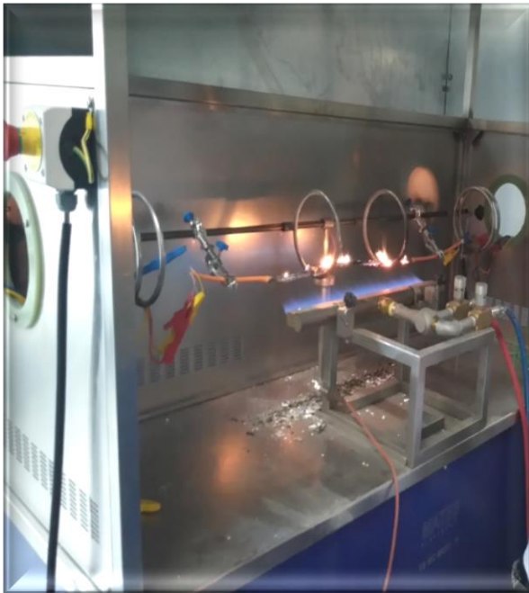
IEC 60331-21: Tests for Electric Cables under Fire Conditions-Circuit Integrity
